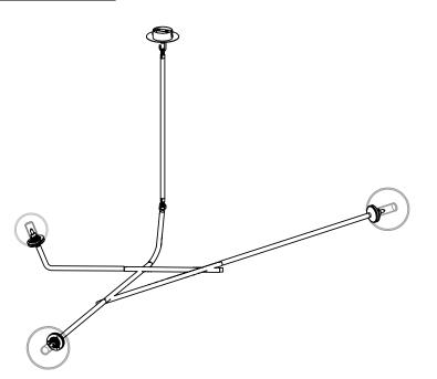
BULB TYPE G9 Eco Halogen bulb Maximum 18 watt
