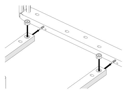
e) Tighten the connections firmly with an Allen Key.
